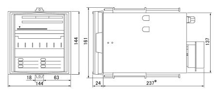
\* 243mm for adding Form A mechanical relay
